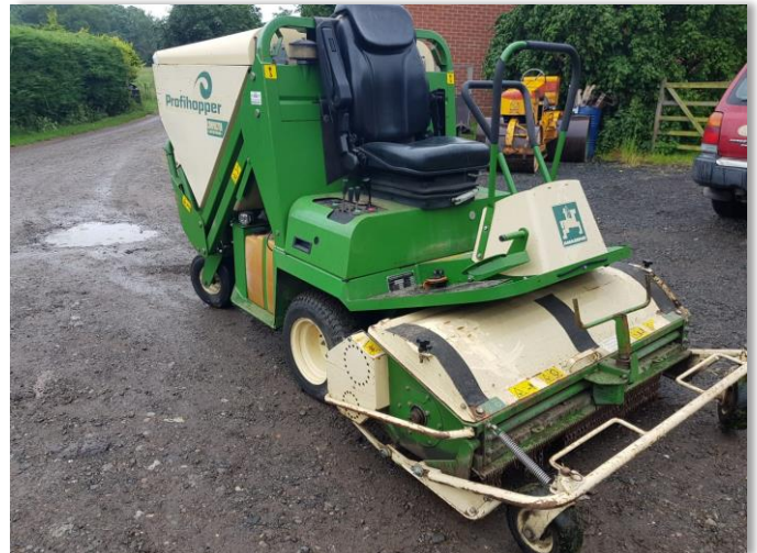
Haydn's Amazone ProfiHopper, ideal for orchards and smaller meadows, can cut, scarify and collect
