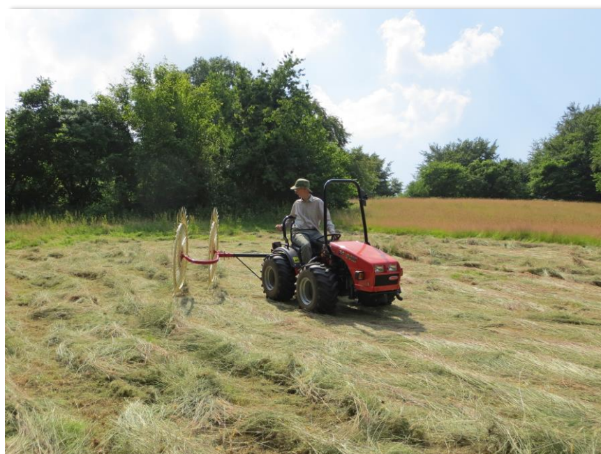
Our Goldoni tractor with tedder attached, perfect for slopes and small areas of land
